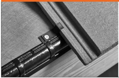
At the eaves the tile clips can be cut short and clout nail fixed through the hole in the face of the clip arm, ensuring that there is a minimum 20mm of penetration into the timber fascia board.
