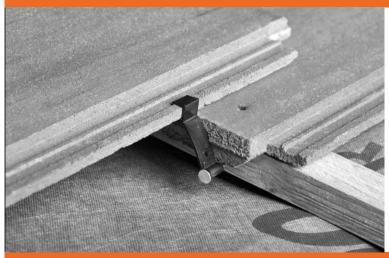
The **Natural Range Tile Clip** is clipped onto the interlock of the tile and then fixed into the batten below using a 65mm x 3.35mm aluminum clout nail (not supplied).
